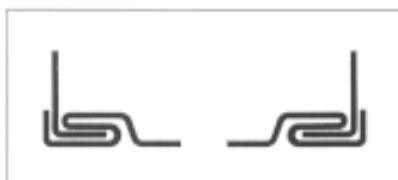
Scroll and side plates, assembled with Pittsburgh seam.
